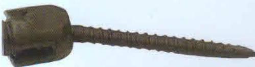
Polyaxial Lateral Mass Screw Mat:- Titanium Cat No.: SPI-LMS-3510-34 Dia:- 3.5 MM Length : 10-34 MM
